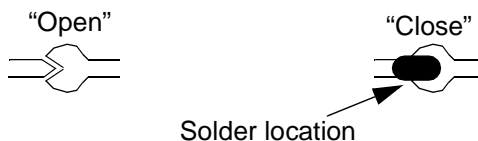
Figure 2-9. Solder Straps location
